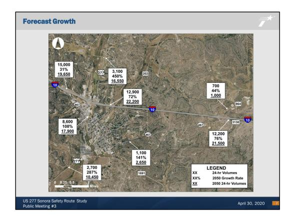
Traffic forecasts for the study area were developed using statewide traffic growth from TxDOT's computerized statewide traffic forecasting model, and a local traffic model of Sonora developed especially for this study.
