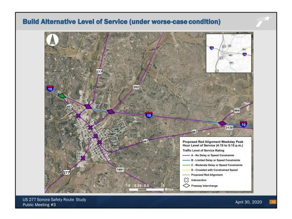
This map illustrates the year 2050 level of service results under the Red alternative illustrated by the dotted line through the west Loop 467 interchange at I-10.
