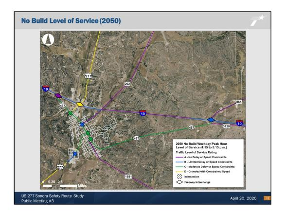
The traffic effects of the relief route were measured by comparing the no build alternative to the worst-case alternative for the relief route, which is the Red alternative.
